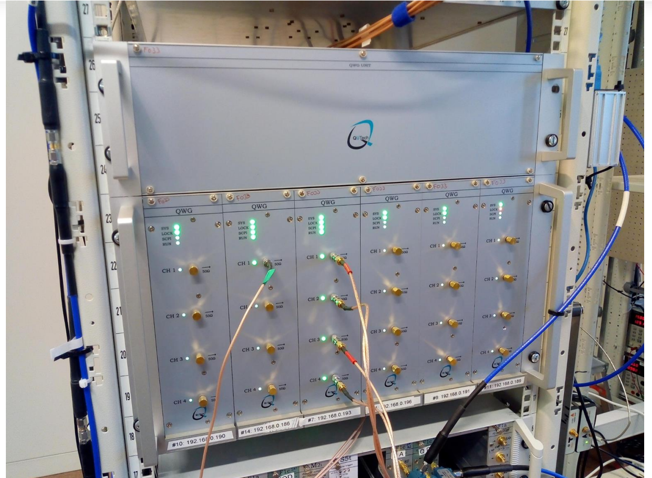
QuTech Waveform Generator (2017) 24 channel AWG in 9U rackspace
